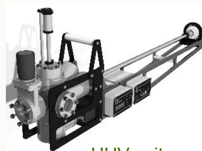
UHV suitcase for sample transfer to other instruments
