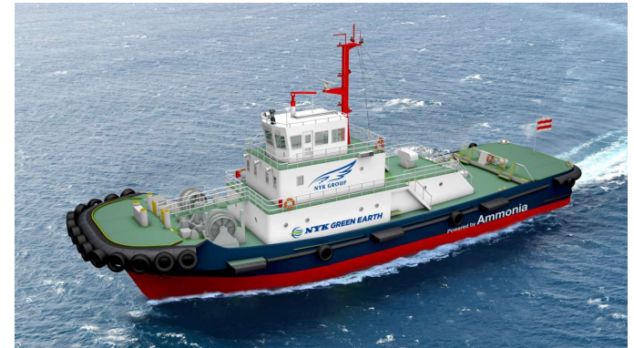
Design of the A-Tug ammonia powered tugboat set to operate in Japan (source: NYK)
