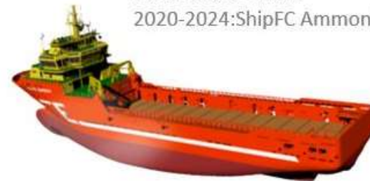
Viking Energy with ammonia-driven fuel cell – Eidesvik
