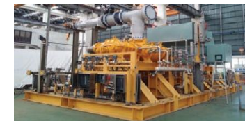
Propane Refrigeration Compressor - Korea 4032XLLLC / 3000kW
