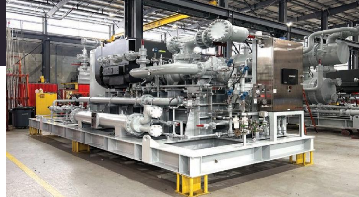
Refrigeration Package - Mayekawa USA 3225SSC / 1000HP
